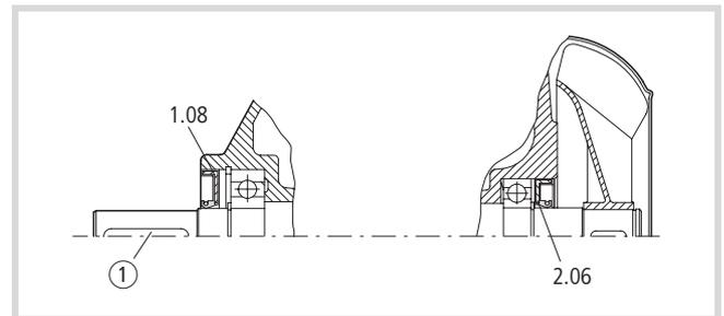
Figure 28: Shaft seal
