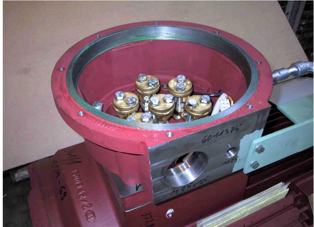
Standard metric threads acc. to catalogue for cable inlets. Exd-cable glands on request only
